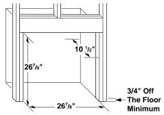
Figure 5 - Rough Opening for Installing in Wall
